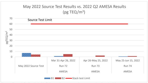
Note 4: Run 73 Boiler Unit #1 (B1) not shown; sample compromised at the lab.
