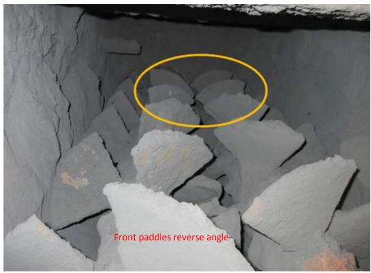
Photo 42 - Double Shaft Mixers – Some Paddles out of Proper Orientation Front Paddles (under rotary) are reversed angled – reported to be by design
