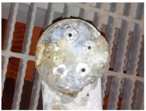
Photo 31 - Spray Nozzle – 3 of 5 Nozzles Plugged – PM Program Lacking
