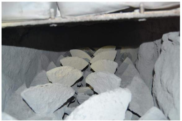
Photo 41 - Double Shaft Mixers – Some Paddles out of Proper Orientation
