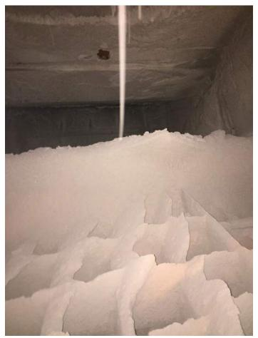
Photo 30 - Vanes at Discharge of Quench Reactor - some Buildup - Not Considered Excessive
