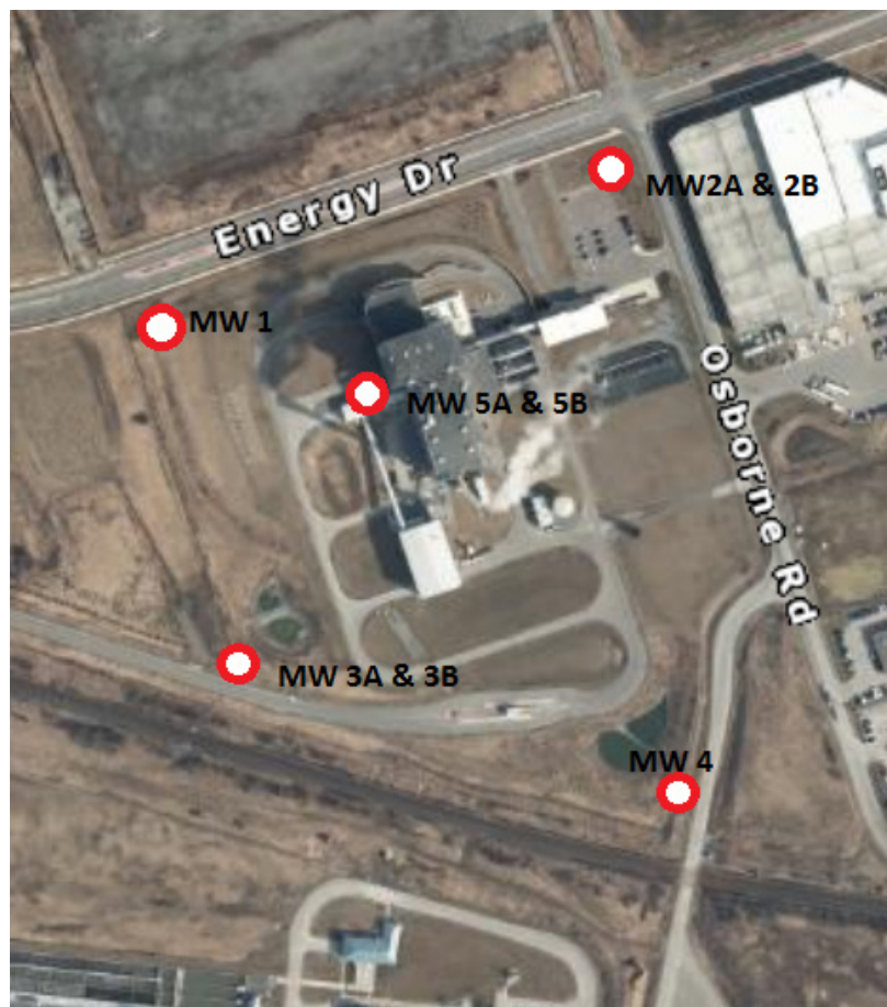
Figure 1: DYEC Monitoring Well Locations
