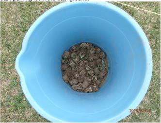
**Photograph-4**: View of a composite sample before being placed the laboratory supplied jars.
