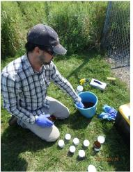
**Photograph-6**: View of WSP field staff sampling at the downwind location.
