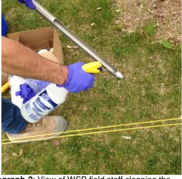
**Photograph-2**: View of WSP field staff cleaning the sampling probe between sample locations.
