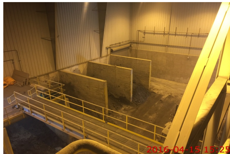
Photo 24: storage of treated ash in bunkers prior to off-site shipment.
