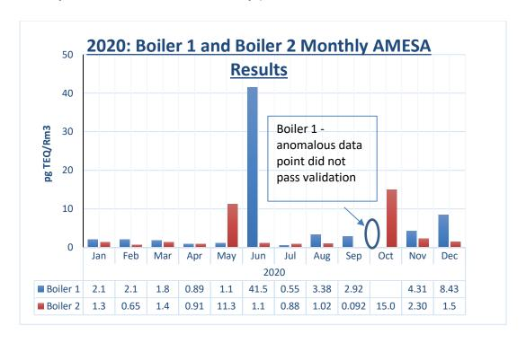
The superior level of compliance (well below the LoQ) contributes significantly to the difficulty of establishing a correlation between the compliance test results and the results measured by the AMESA system to BSI CEN/TS 1948-5 standards.
