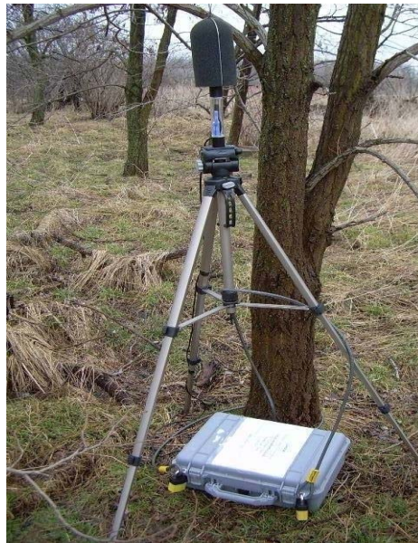
Figure 4-2 Ambient Sound Level Meter Set-Up
